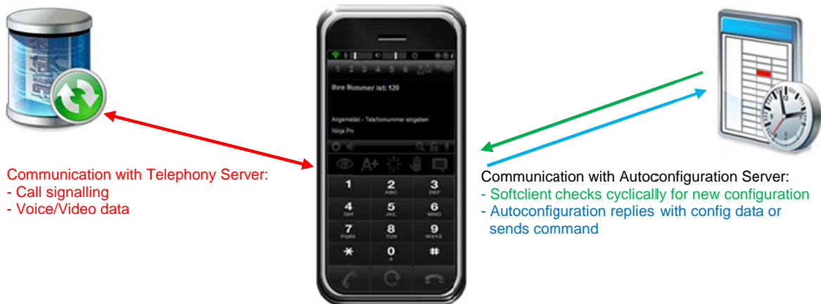
Fig. 3: Ninja Enterprise repeatedly checks on the autoconfiguration server for new configuration data
